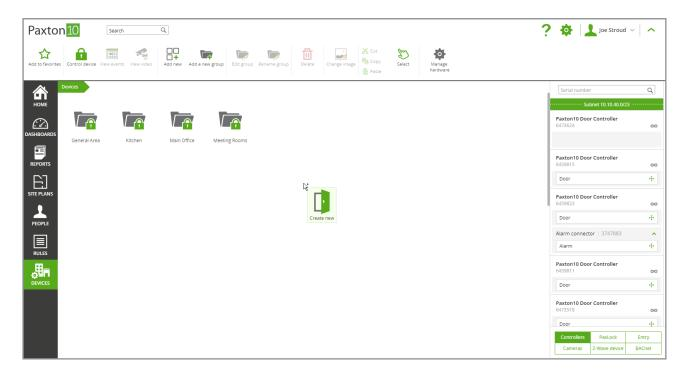
Once a component from the Paxton10 controller is mapped to a device in Paxton10, the controller is then bound to that Paxton10 system, and can't be detected or controlled by any other system.
